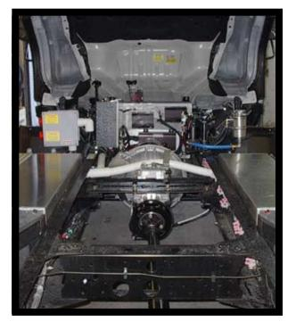
The FMI Isuzu Electric Drive system was specifically designed for airport ground support equipment (GSE) applications. The electric vehicle has a GVWR of 12,000 or 14,500 lbs. and a top speed of 25 MPH (40 KPH) forward, 7 MPH (11 KPH) reverse, along with a traveling distance from 17 to 35 miles (27 to 65K) between charging. Opportunity charging can dramatically increase maximum daily mileages. The unit is ideal for GSE applications.
